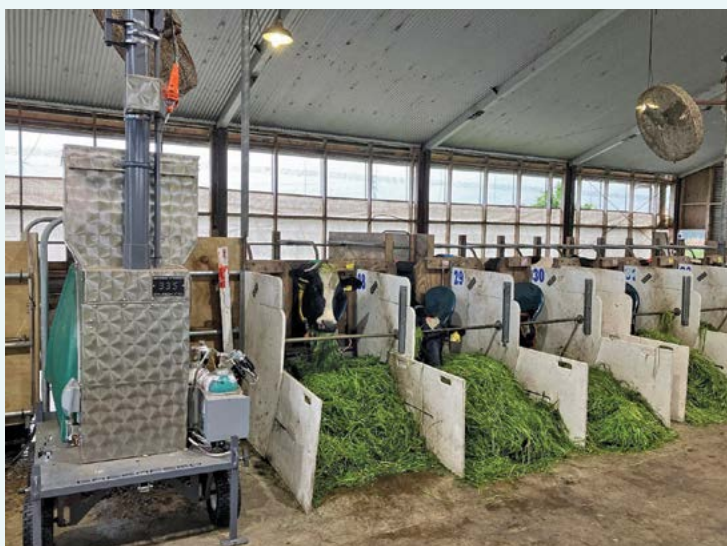
Using a Calan gate system enables our researchers to measure feed intake and methane from lactating cows fed pastures over time.
