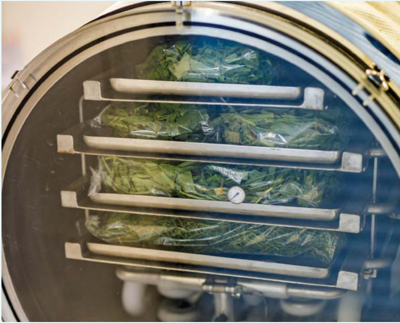
Pasture samples being freeze-dried before being ground and sent for lab assessment. This method is more effective than oven drying to preserve sample quality.
