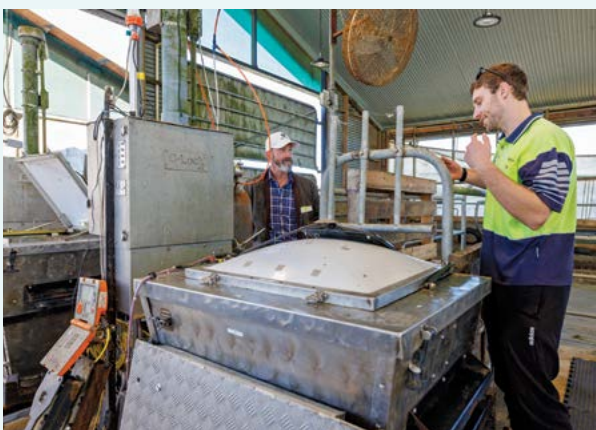
DairyNZ research technician Addam Knight (right) demonstrates the GreenFeed/SmartFeed unit that measures methane and cow intake.
