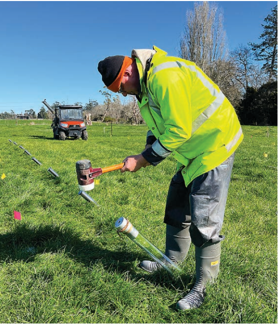
Senior Research Technician Adam Benton installing rhizotrons to study how pasture management above ground affects root growth and pasture persistence.
