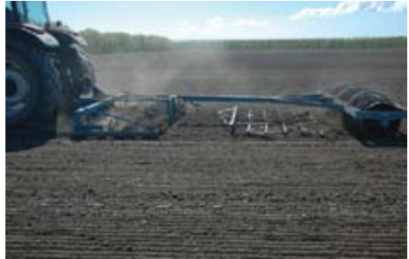
Consolidation using tyne harrows and a Cambridge roller is highly recommended.
