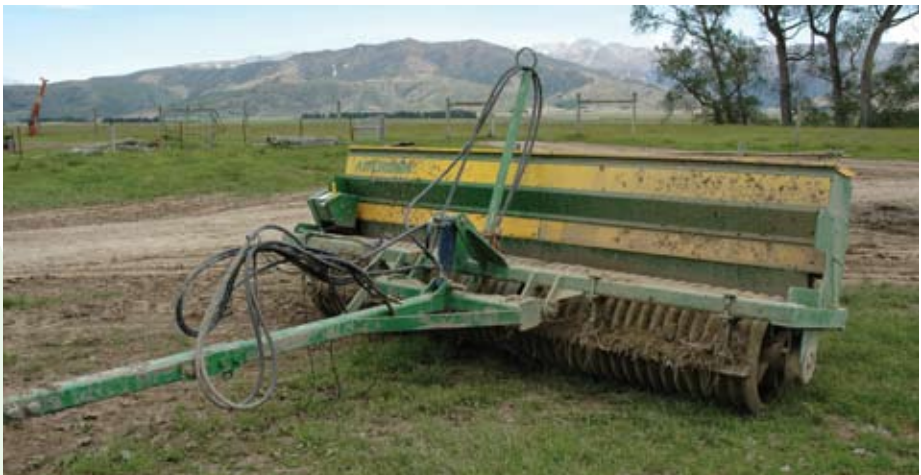
A Cambridge or specialised rung-type roller with a seed box fitted to the back.
