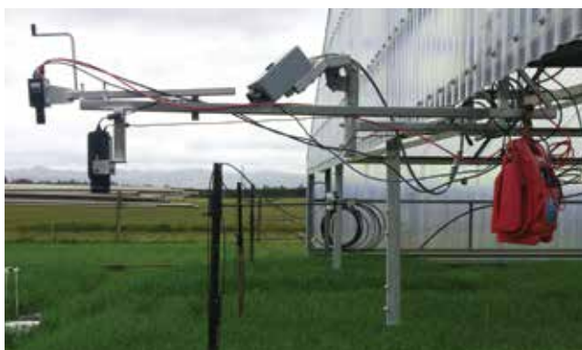
a) Sensors mounted onto the Plant & Food Research Lincoln rain shelter.
