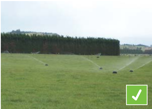
Systems operating at the correct spacing and layout to deliver good application depths and a uniform spread.
