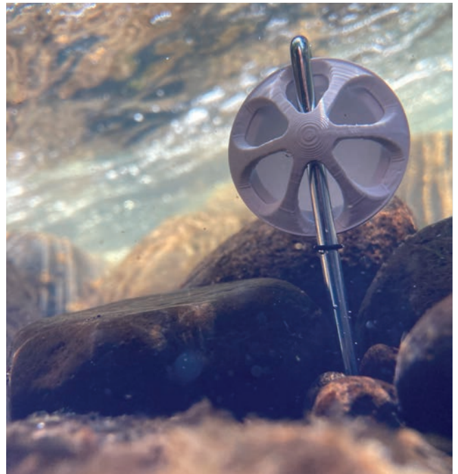
Farmers can use this simple water sampling tool to collect eDNA. Samples are then sent to a lab for analysis, to provide an overall estimate of stream condition.
